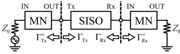
Fig. 4 Condition of simultaneous matching for a SISO system.
