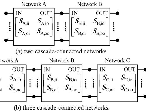
Fig. A·1 Cascade-connected multiple networks.
