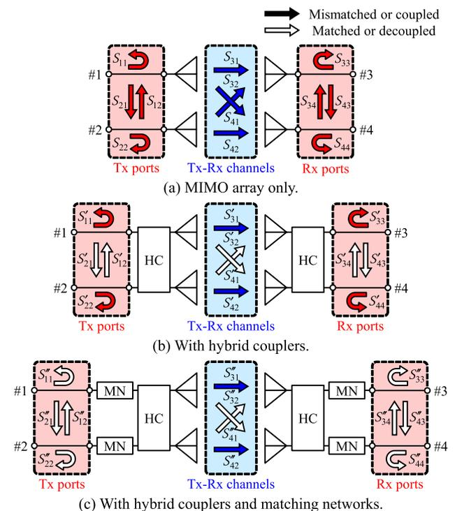
Fig. 3 Conceptual diagram of the S-parameter on each stage.
