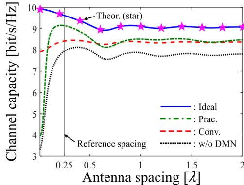
Fig. 11 Channel capacity versus antenna spacing.
